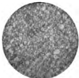
Fig. 4.—Marble, Carrara, Italy A section of well-known statuary marble which consists entirely of calcite in small irregular crystals closely fitted together.
