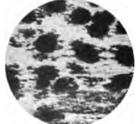
Fig. 6.—Obsidian, Iceland. In the clear glassy base there are rounded, yellow spots (spherulites) arranged in fluxion streams.
