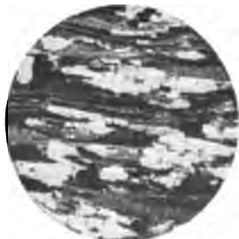
Fig. 8.—Mica-Schist, Blair-Atholl, Perthshire, Scotland. A clay rock like the preceding one, but more metamorphic and coarsely crystalline. The clear spots are quartz and the bladed mineral between them is brown and white mica (biotite and muscovite).
