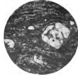
Fig. 9.—Porphyritic and Fluidal Rhyolite, Hungary. The ground mass is partly glassy, partly felsitic, and shows fluxion-banding. The large quartz is a double hexagonal pyramid, but its edges and corners are rounded by corrosion and large irregular areas of glass penetrate to its centre.
