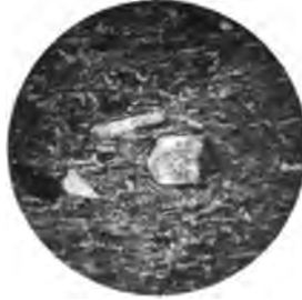
Fig. 2.—Fluidal Rhyolite, Hungary. In the centre are crystals of feldspar, rather turbid through weathering. The matrix is partly glassy, partly felsitic, and shows the effects of streaming movements with eddies behind the feldspar crystals.
