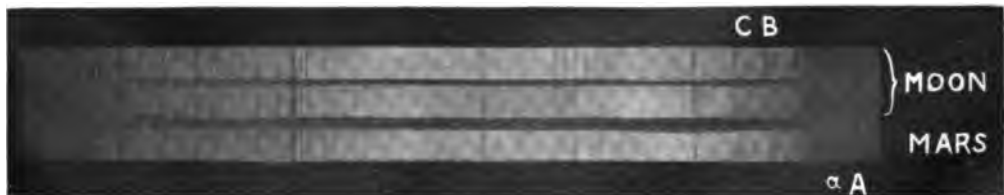
Comparison spectograms of the Moon and Mars, showing absorption bands in that of the latter, which denote the presence of water vapour in the Martian atmosphere (see MARS).
