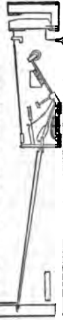
FIG. 29.—Wornum's Upright Action, 1826. The original of the now universal crank action in upright pianos.
