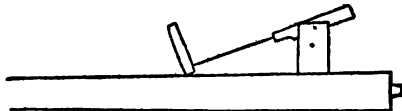
FIG. 20.—Old Piano Action on the German principle of Escapement. Square Piano belonging to M. Gosselin, Brussels.
