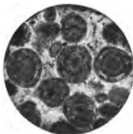
Fig. 5.—Oolitic Chert (Cambrian), Sutherlandshire, Scotland. This has been once an oolitic limestone, but the calcite has been entirely replaced by silica with perfect preservation of the oolitic structure.
